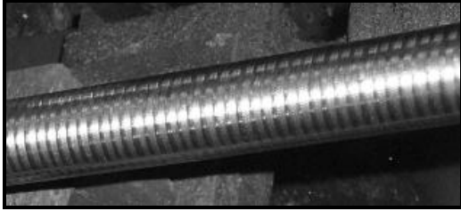
Fig. 8 Ringing pattern on bright bar (RCMX 2507 MOS50-R50)
