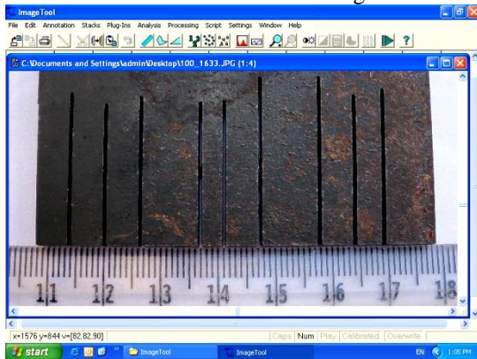
Fig. 4 Print screen of image tool software measuring Kerf width
