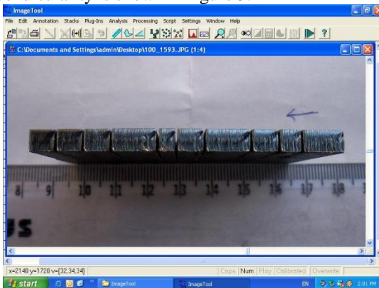
Fig. 5 Print screen of image tool software measuring Perpendicularity
