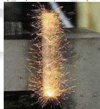
Fig. 6: Photo of dry HS-WEDM (Wang, T., (2011))
