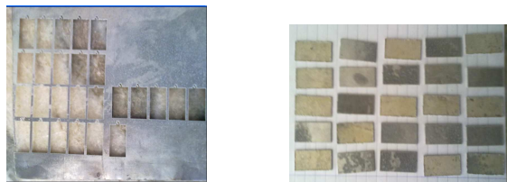
Figure.1 Specimen after Machining (Aluminium): Size –400X500mm and Thickness 1mm
