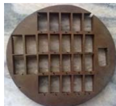
Figure.1 Specimen after Machining (En 8): Size - Dia.170mm and Thickness 10mm
