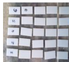
Figure.3 Specimen after Machining (aluminium): Size –400X500mm and Thickness 4 mm
